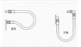
当弯曲半径太小时,宜采用直角接头以免胶管出现急弯。 Choose right angle fittings to avoid too small bending radius and excess force,
