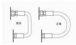
为避免胶管被破坏及流量受限制,胶管弯曲半径应尽可能加大。 Hose bending radius should be as big as possible when it is in motion.
